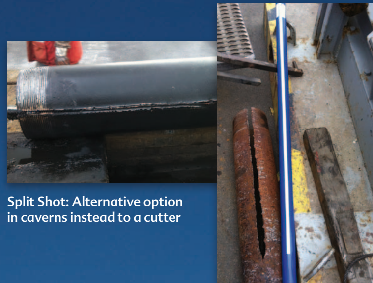
Use of a Severing Tool to recover a stuck 5 1/2" drill pipe
