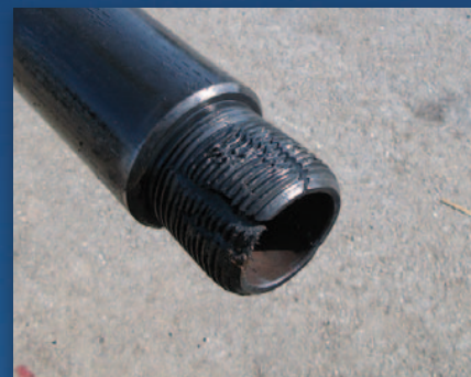
Use of a Severing Tool to recover a stuck 5 1/2" drill pipe
